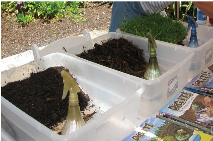
From left to right bin 1 has bare soil, bin 2 has soil with mulch covering it, bin 3 has soil with grass cover. Each were sprayed with the same amount of water (rain). As expected the bin with bare soil had more and muddier “runoff” at the end of the day.
